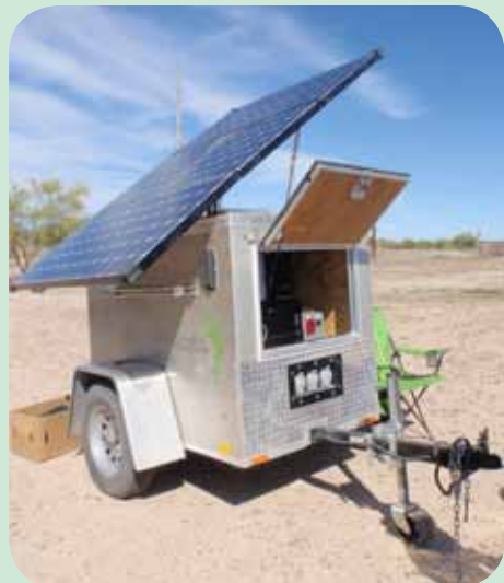
We produced our own electricity using this trailer, which was hauled by our gear truck.
